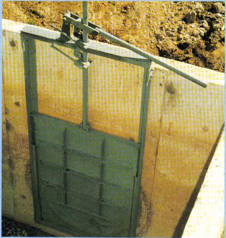
Low Head Jack Gate fabricated from 3.2mm material suited for water diversion. Quick operation and economical. This valve is 900mm and was grouted in after head wall construction. Suitable for water diversion purposes with head pressure of 0.6m above the incoming pipe.
